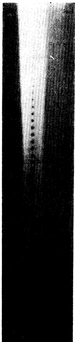
Fig. 5. Photograph of Burning Droplet Array(n-dodecane, 1000 K, 50% O 2 , 10 KHz, initial dia. = 180 \mu m)
