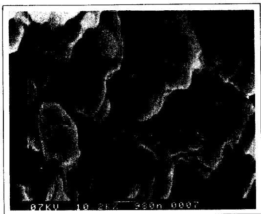
Fig. 8. Inner-structure of the sulfonated membrane 30 wt% DVB, SR=0.5 ( \times 10, 200 ).
