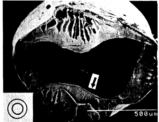
Fig. 24. Crosssectional view of 18wt% polysulfone membrane ( \times 100 ). PVP(M.W. 10,000) 15%, DMA Solvent, Air gap: 105 cm, \uparrow : crack
