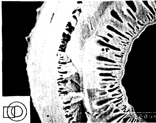
Fig. 13. 35wt% polysulfone HF membrane. PS/DMA = 35/65, Bore coagulant : water
