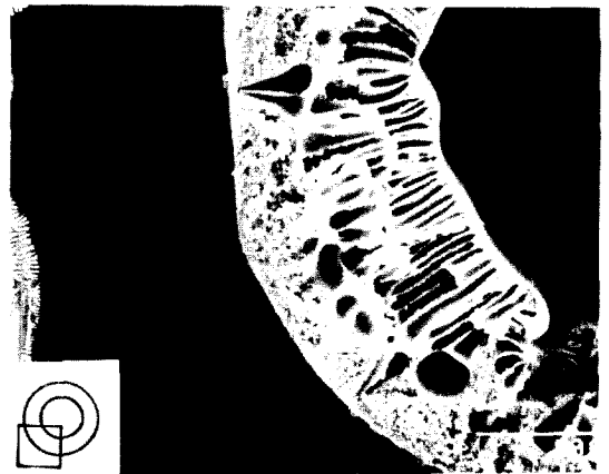
Fig. 11. HF membrane spun with 98wt% IPA + 2wt% water as bore coagulant. PS/DMA/PVP = 18/67/15
