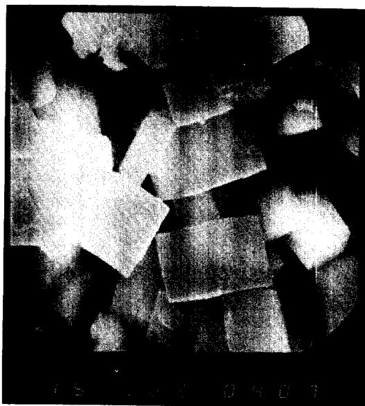
Fig. 2. Scanning electron microgram of the H-ZSM-5 ( \times 10^4 ).
