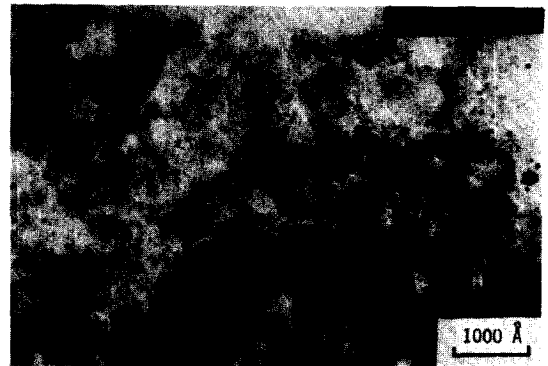
Photo. 2. Transmission electron micrograph of Pt (0.5 mg/cm²) on Vulcan XC-72 (×100k).
