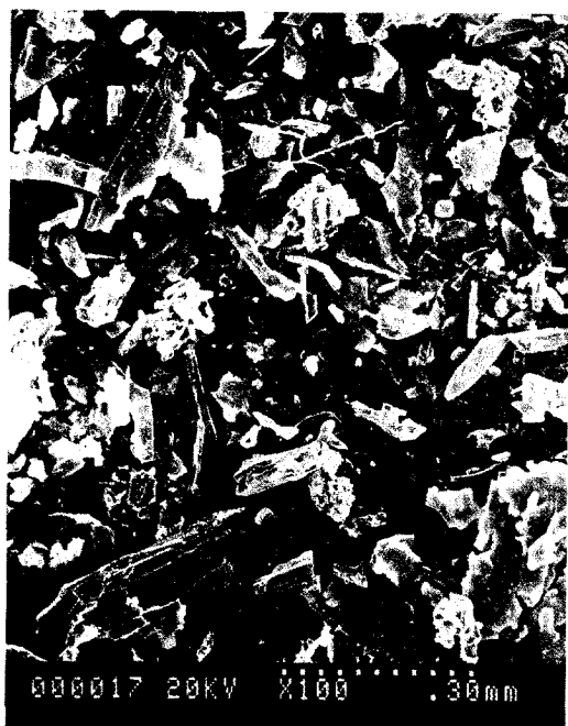
Fig. 4. Scanning electron microgram of \text{MoS}_2 prepared at 450^\circ\text{C} .
