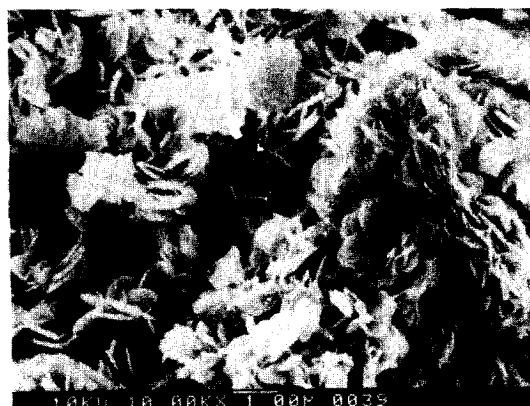
Fig. 2. Electron micrograph of V 2 O 5 -P 2 O 5 catalyst.
