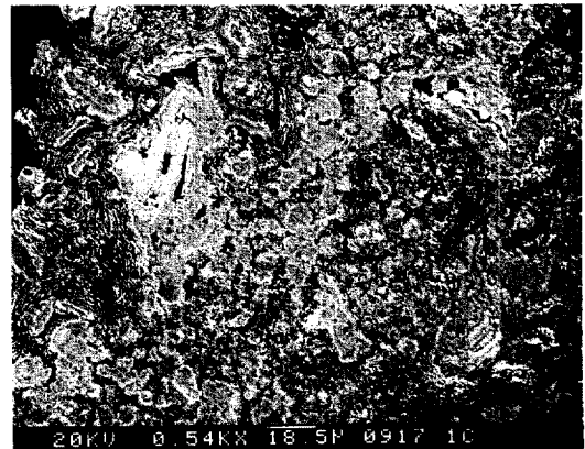
Fig. 9. Microstructure of PAM made from lead oxide after formation.
