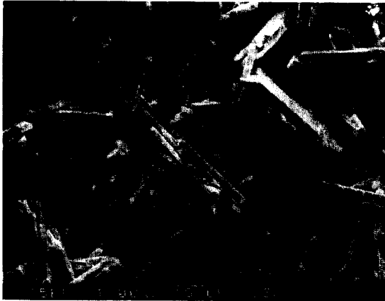
Fig. 2b. SEM micrograph of tetrabasic lead sulfate.
