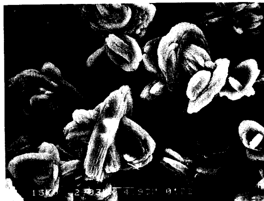
Fig. 3. Scanning electron microscope photograph of hydrothermally synthesized Ti-Al-mordenite.
