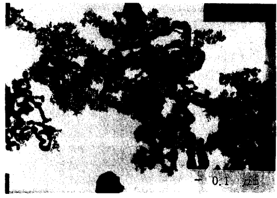
Fig. 6. Transmission electron microscopic image of Fe-Co ultrafine powder produced under the condition of cooling.
