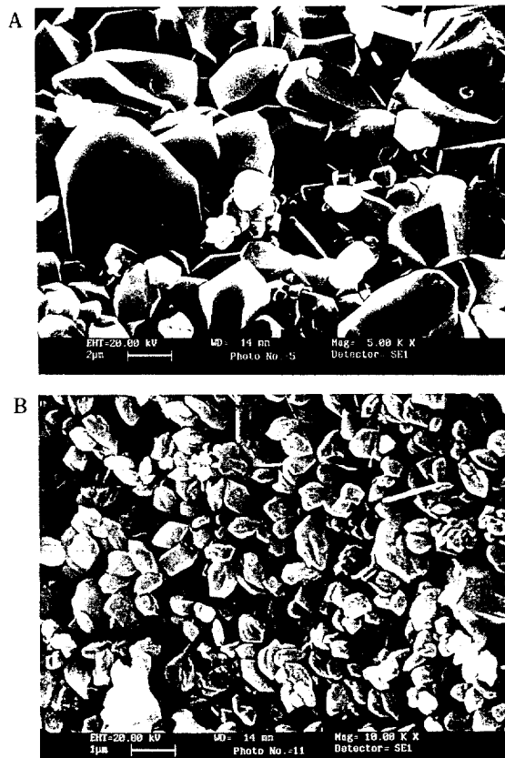
Fig. 7. SEM micrographs of \alpha -SiO 2 powders formed by the hydrothermal reaction using 0.5 wt% seed crystal powders for 3 h reaction at 400 °C. (A: with 0.1 wt% KOH, B: with 1.0 wt% KOH).
