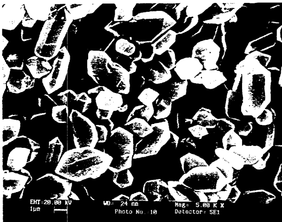
Fig. 9. SEM micrograph of \alpha -SiO 2 powders formed with 0.8 wt% KF by the hydrothermal reaction using 0.5 wt% seed crystal powders for 3 h reaction at 400 °C.
