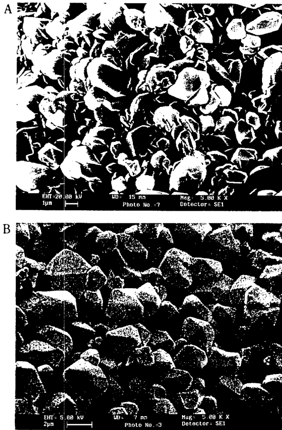
Fig. 8. SEM micrographs of \alpha -SiO 2 powders formed by the hydrothermal reaction using 0.5 wt% seed crystal powders for 3 h reaction at 400 °C.
