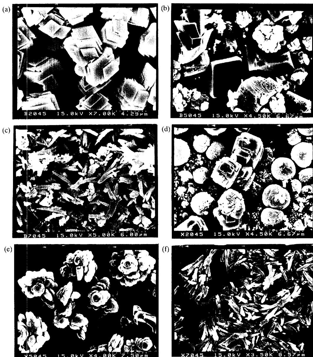
Fig. 4. Scanning electron microscopy of calcium carbonate in bulk-mixing-reaction.
