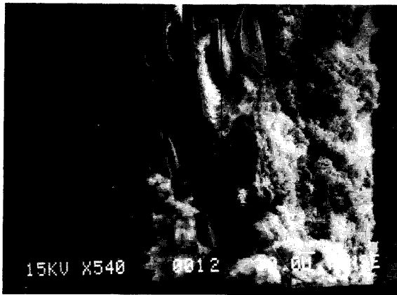
Fig. 5. SEM photograph of the electrode including ACF(cross section).
