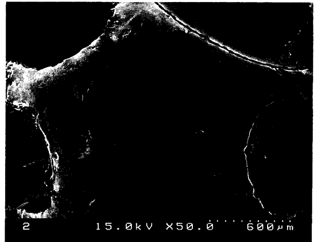
Fig. 2. Scanning electron microscope for the deposit of electroless nickel plating on poly-urethane substrate.
