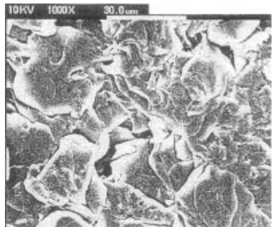
Fig. 16. Shape of polypropylene extracted from bioriented films by scanning electron microscopy(magnification 1,000).
