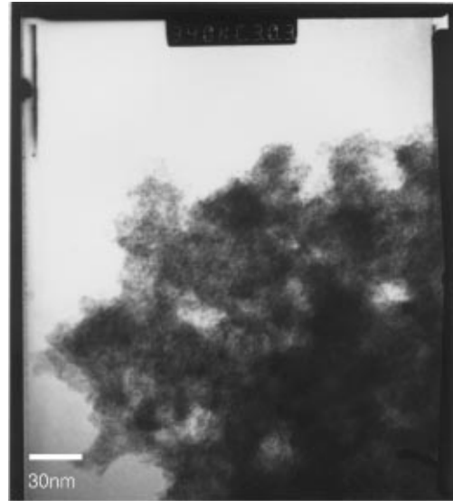
Fig. 5. TEM image of 1.5 YSZ powder dried at 100 °C.
