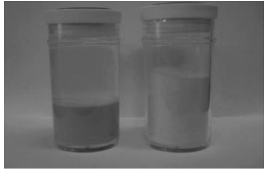
Photo 1. Configuration of cerium hydroxide(III) and (IV).
