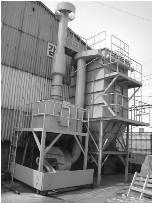
Fig. 16. The picture of system for removing simultaneously dust and VOC.
