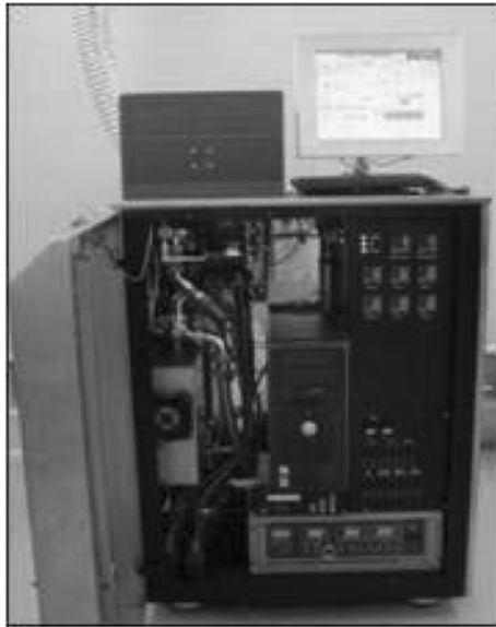
Fig. 3. Automatic Vapor SAM coater for release layer.
