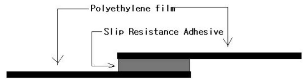
Fig. 2. Image of 180° peel test specimen.
