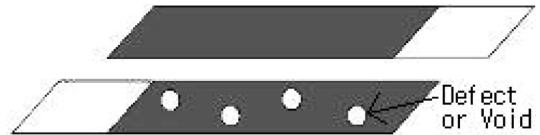
Fig. 3. Cohesion failure.
