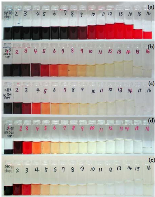
Fig. 7. Changes in colour during the catalytic wet oxidations of RB5 with the CuO concentrations of (a) 0.00 g/l, (b) 0.01 g/l, (c) 0.02 g/l, (d) 0.05 g/l, and (e) 0.20 g/l at 190 °C; Sample numbers 1-16 represent samples collected at 1, 5, 10, 15, 20, 25, 30, 35, 40, 50, 60, 70, 80, 90, 105, and 120 min, respectively.
