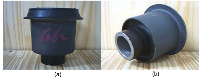
Fig. 1. Torque-rod-bush produced by K company: (a)Front view; (b)Side view.
