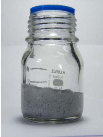
Fig. 3. Photograph of gel formed after \text{NaBH}_4 hydrolysis reaction.
