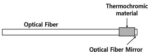
Fig. 1. Optical fiber sensor to monitor temperature.
