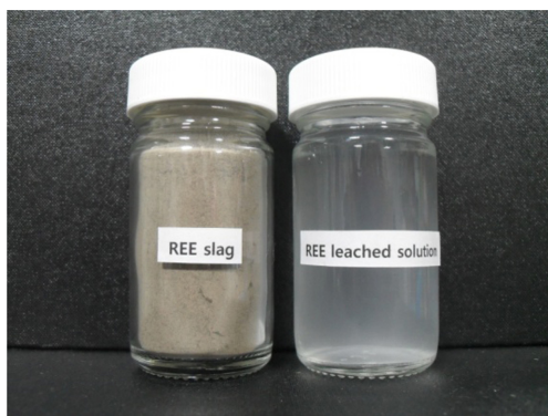
Fig. 5. Photograph of REE slag and REE leached solution.
