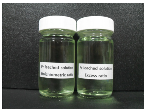
Fig. 4. Pr leached solutions of stoichiometric ratio and excess ratio.
