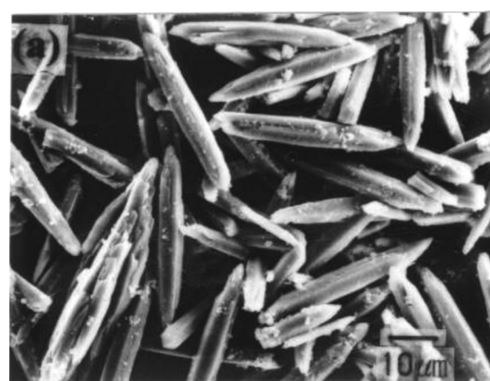
Fig. 3. SEM photographs of aragonite for the conditions in Table-1, batch 4 (Source: Modified figure adapted from reference-42).
