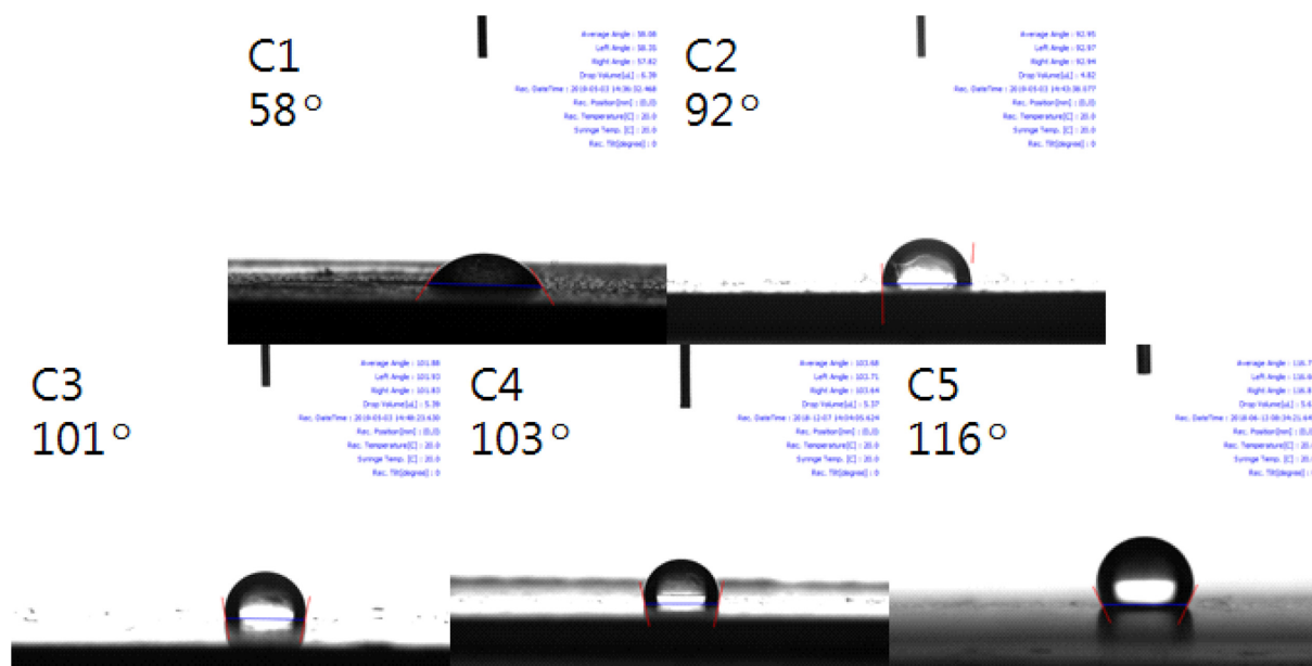
Fig. 6. Contact angles of surfaces of cold-rolled steel sheets prepared with different catalysts in Table 1.
