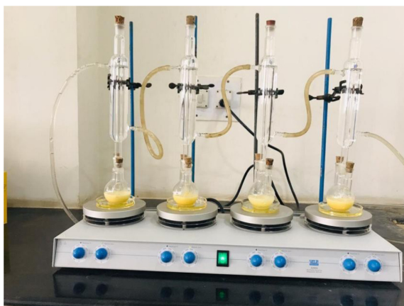
Fig.1. Experimental set-up for the esterification of glycerol.
