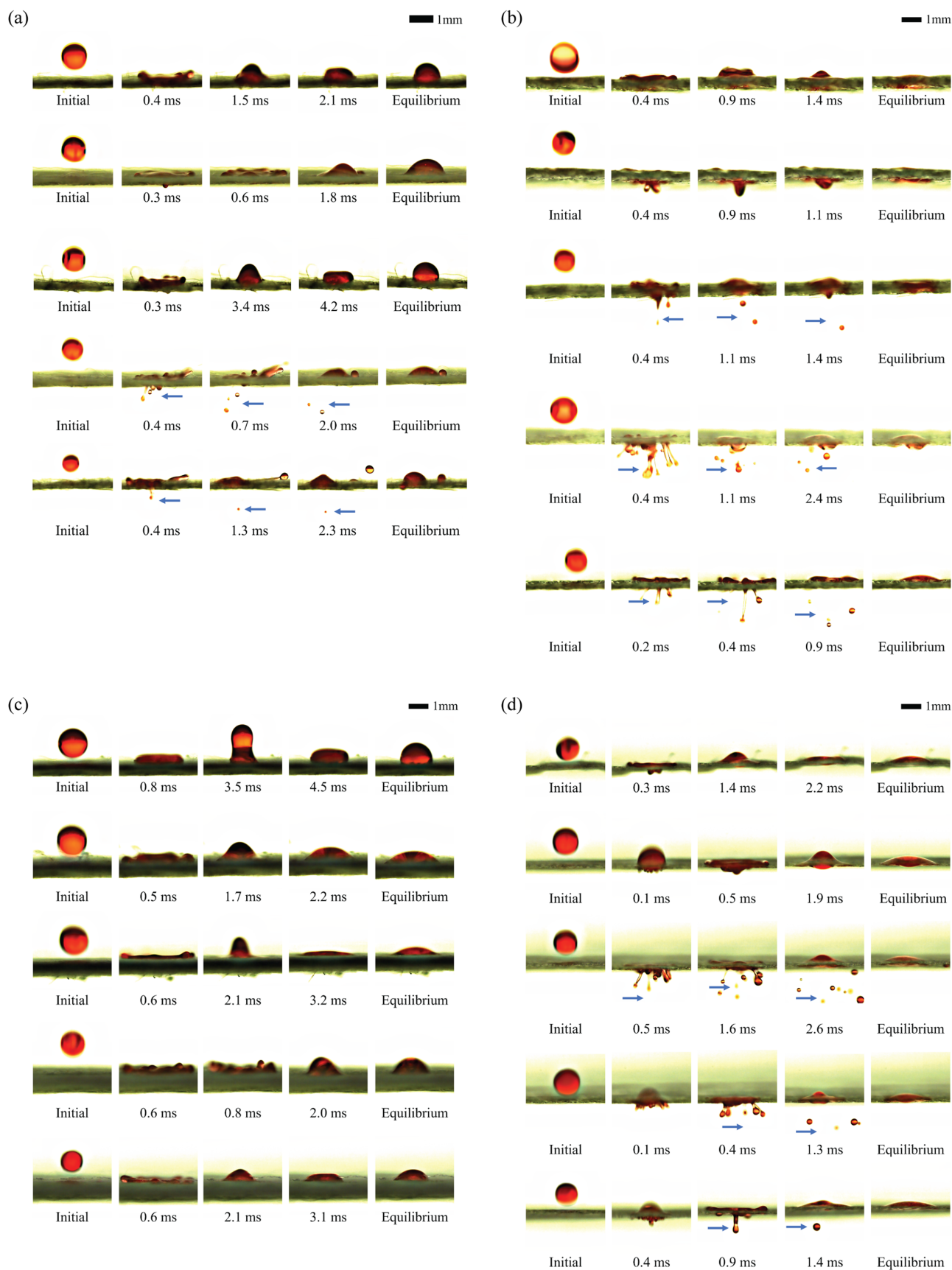
Fig. 4. Consecutive images of droplet impacting dynamics on four filter layers consisting of the KF-94 face mask at different Weber numbers: (a) Layer 1 (i.e., outside layer), (b) Layer 2 (i.e., support layer), (c) Layer 3 (i.e., melt blown filter layer), and (d) Layer 4 (i.e., inside layer). Note that the impacting velocity (i.e., Weber number) increases from the top row to the bottom row of each figure. The blue arrows indicate secondary droplets break up from the liquid filaments.
