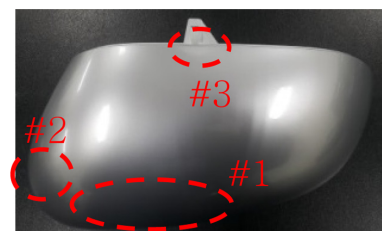
Fig. 9. Paint-free metallic outside mirror housing part.
