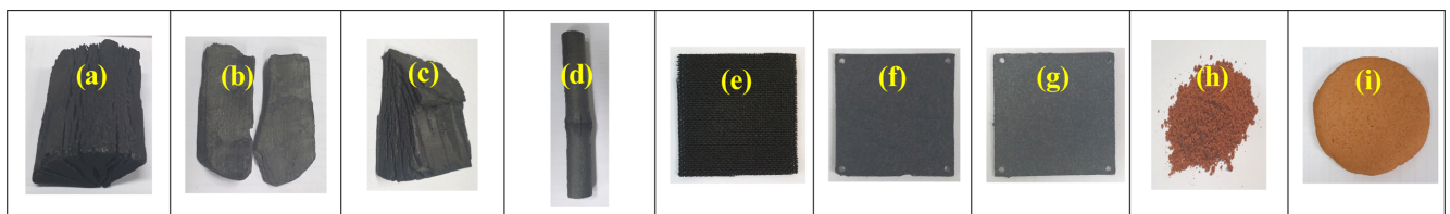
Fig. 1. Charcoals (a: Jincheon, b: Sangrok, c: Anseong, d: Damyang bamboo), (e) ACF fabric, (f) ACF paper(Jiri-san Co.), (g) N-ACF paper, (h) red-clay powder and (i) red-clay cake (Boryeong).
