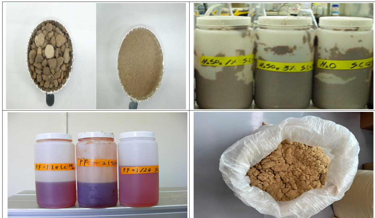
Fig. 1. Images of rapeseed flour (top – left), rapeseed flour hydrolyzates (top – right), phenol-formaldehyde prepolymer (bottom – left) and wood fiber (bottom – right) used for formulating rapeseed flour-based adhesive resins.
