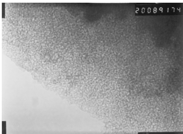
Fig. 2. TEM image of mesoporous alumina, AIS-1, calcined at 420 °C (1 bar: 20 nm).
