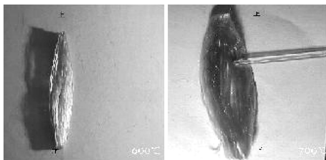
Fig. 10. The cured PCS fiber thermostatically pyrolyzed at 600 °C (left) and 700 °C (right) for 35 minutes (the flow rate of nitrogen is 150 ml/min).
