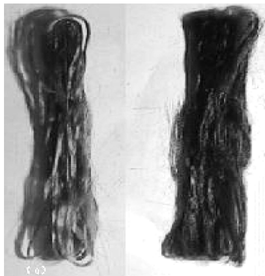
Fig. 12. The photos of cured PCS fibers heat treated at 700 °C (left, in pure nitrogen; right, in nitrogen and offgas).
