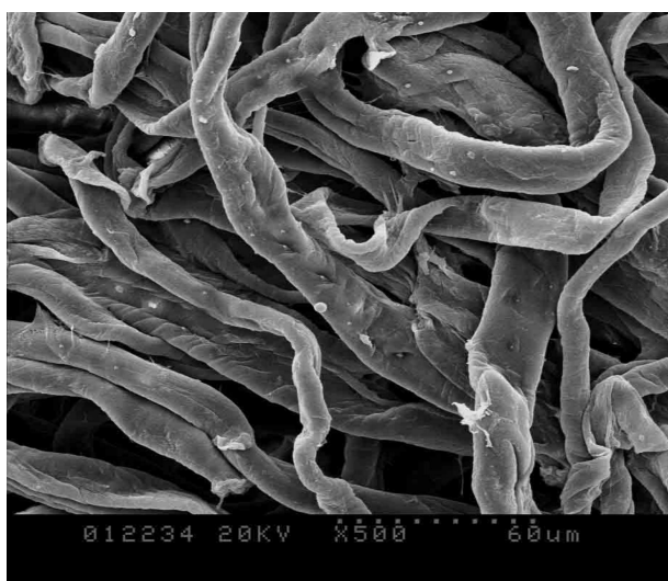
Fig. 5. SEM micrograph of immobilized enzyme.
