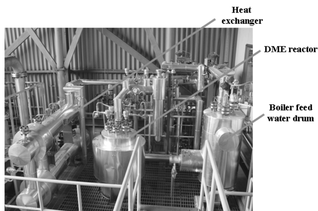
Fig. 3. The DME synthesis system.
