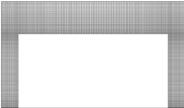
Fig. 2. Mesh structure over the porous material.
