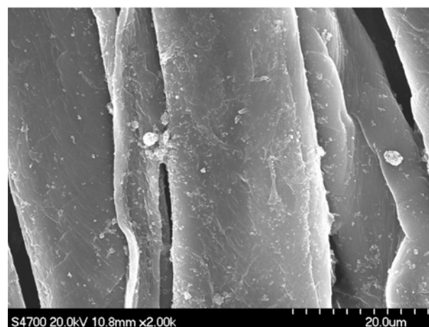
(b) Treated with chitosan/nano-TiO 2 composite emulsion
