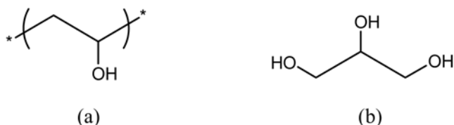
Fig. 1. Chemical structures of (a) poly(vinyl alcohol) and (b) glycerin.
