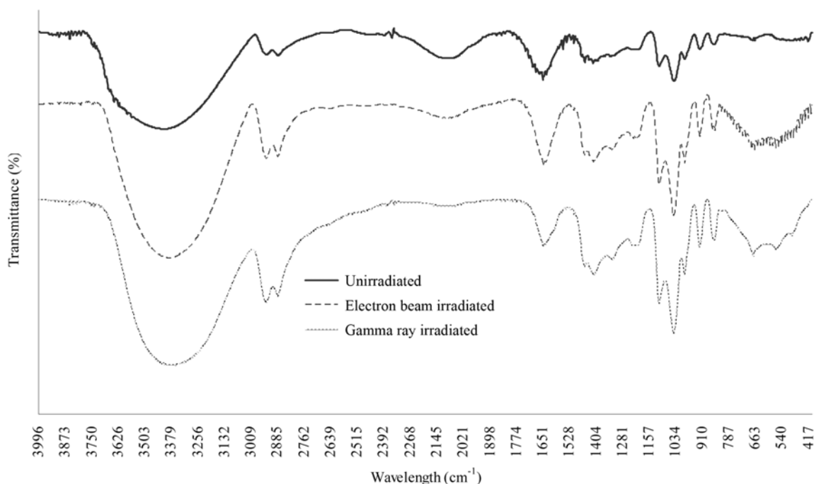
Fig. 3. FT-IR spectra of the unirradiated CMC and the gamma ray- and the electron beam-irradiated CMC samples at the dose of 30 kGy.
