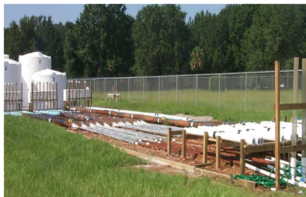
Fig. 1. Pilot distribution system for bacterial regrowth.
