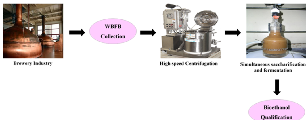
Fig. 10. Waste from beer fermentation broth is evaluated for bioethanol production via SSF at gradually increasing temperatures from 25 °C to 67 °C during culture at 150 rpm.
