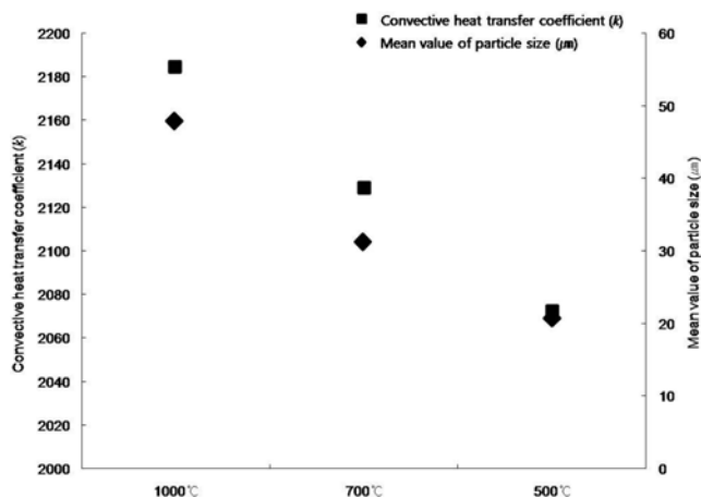
Fig. 8. Variation of convective heat transfer coefficient and particle size of coal fouling by deposited temperature (Centennial coal).
