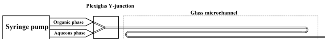
Fig. 1. Y-channel design of the microchannel.
