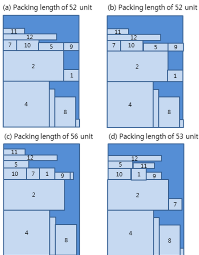
Fig. 8. Comparing this strip packing method with previous methods for the example reported by Ntene et al. [10]. (a) Our strip generation algorithm (b) The knapsack algorithm [5] (c) The next-fit decreasing height algorithm [8] (d) The first-fit decreasing height algorithm [8].
