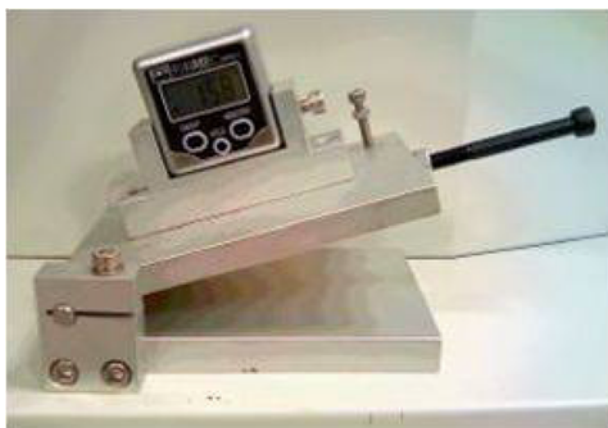
Fig. S1. Photograph of sliding angle measurement system equipped with digital angle meter.
