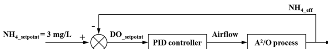
Fig. 2. Control loop based on the effluent \text{NH}_4\text{-N} concentration.
