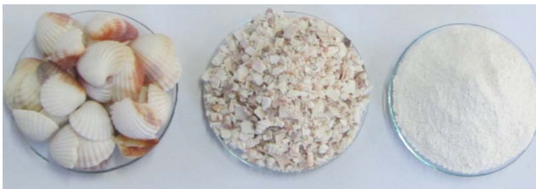
Fig. 2. The images of scallop shell sample: (a) natural scallop shell, (b) ground sample using a hammer mill, (c) powdered sample in the size range of 50 meshes ASTM.
