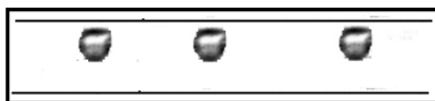
Fig. 7. Bubbly flow observed U_g=0.3 m/s, U_l=0.9 m/s and the part of image obtained after processing in 2.6 mm tube.
