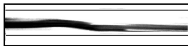
Fig. 20. Stratified wavy for U_g=7.85 m/s and U_l=0.04 m/s for and the part of image obtained after processing in 2.6 mm tube.
